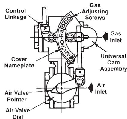
Having marked and/or recorded the MICRO-RATIO® Control Valve's air valve settings for both minimum and maximum firing positions, you may adjust the linkage and travel of the gas valve's stroke (see sketch below).
