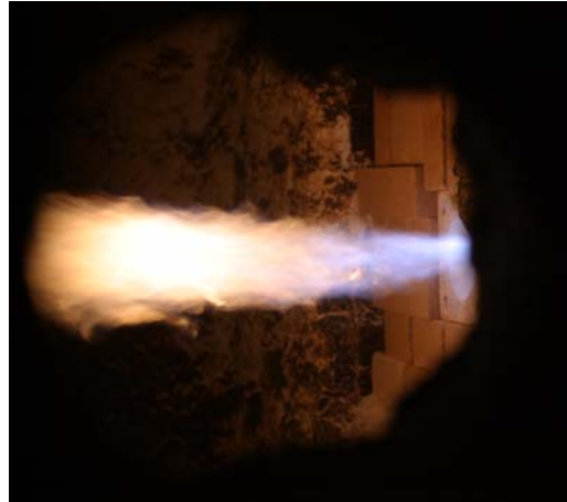
OXY-THERM® LE staged flame pattern
