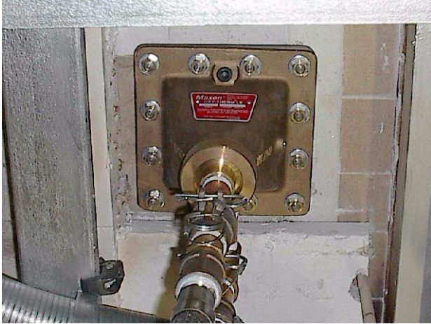
OXY-THERM® LE mounted on a glass furnace
